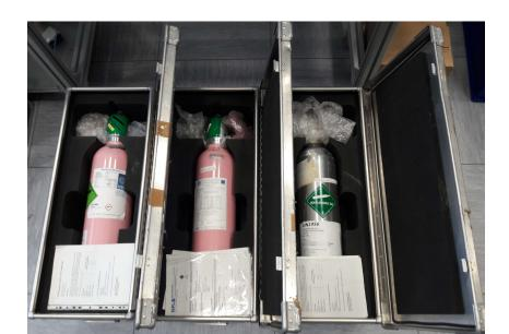
1 x NPL NMHC Standard (4 ppb in N<sub>2</sub>) 2 x NMHC Mixtures in amb. Air
