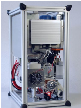
Photo: https://www.tesscorn-aerofluid.com/ Filter absorption photometer Proton Transfer – Mass Spectrometer (PTR-MS) volatile organic compound concentrations
