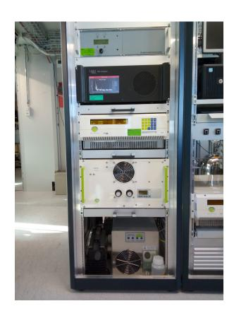
NO with chemiluminescence (Ecophysics) NO2 with laser spectroscopy (Miro Analytical)
