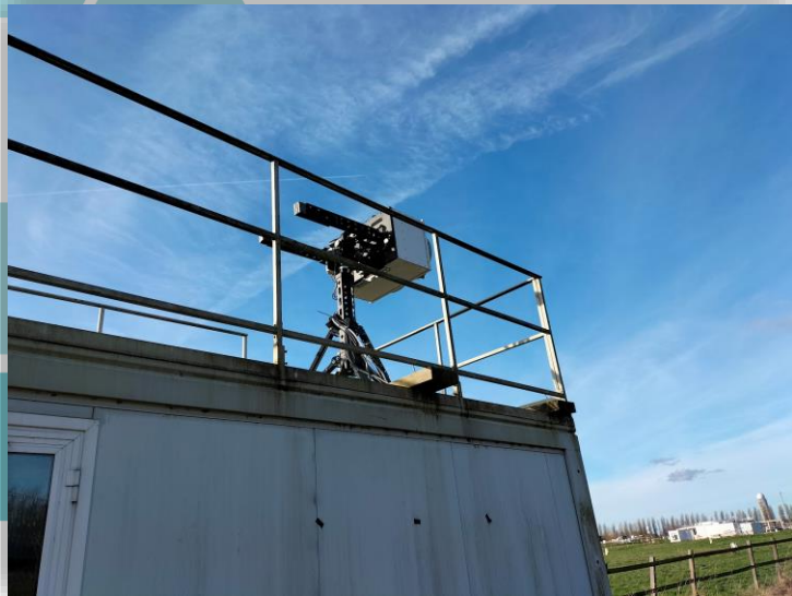
BASTA-Mini CCRES aiming at a 10 cm Corner Reflector 376 m away
